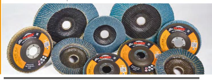
Thanks to the fiberglass backing pad, these flap discs cannot pollute the surface worked; while this occurs during grinding operations with discs having a plastic backing pad. This phenomenon can occur once the abrasive cloth is used: for this reason flap discs with fiberglass backing pad are especially suitable for working stainless steel.
