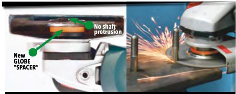
Thanks to the use of the special **"SPACER"** and to the depressed center shape, the machine shaft and the locknut do not extend from the dome cavity thus enabling the operator to carry out flush cuts in a comfortable and safe position. The depressed center shape gives more rigidity than a flat disc, prevents bending allowing to make perfectly straight cuts.
