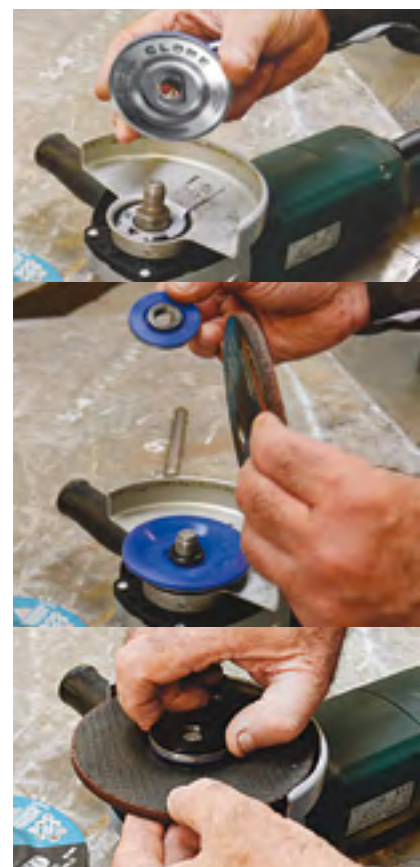
VIBLOCK is quick and easy to assemble. (photos above), and mounts only on Globe Type 27 discs. On the left VIBLOCK on a Globe Ceramic Power 'CD' disc.
