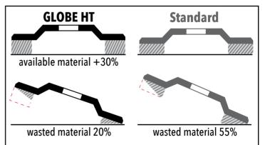
A disc of 'high thickness'. The different compactness and relative advantages between a Globe HT flap disc and a standard disc.
